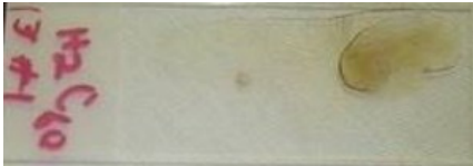
Glass Slide with a spot made from buckyball solution
